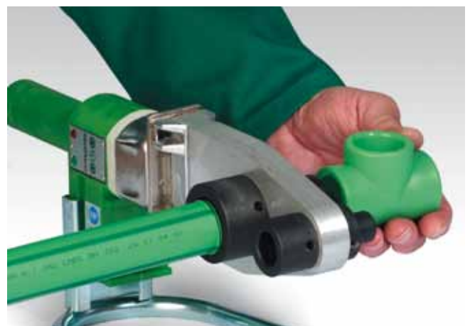
Heating-up of pipe and fitting
