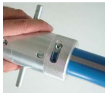
Peeling of the oxygen barrier layer
